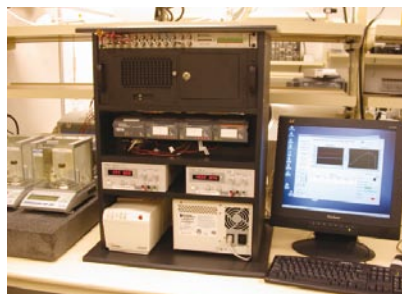
Figure 2. Stroke volume test system uses PXI and FieldPoint to collect data and control temperatures
